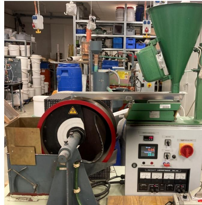
Low Intensity Magnetic Drum Separator (LIMS)\*
