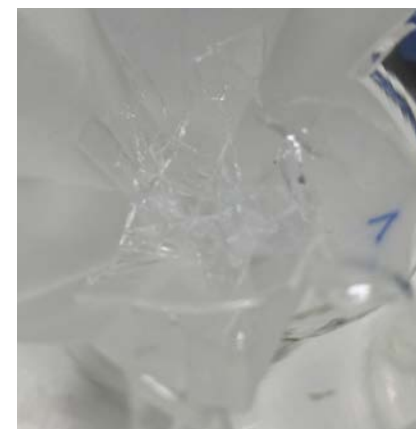
Damp heat treated BPO after solvation experiment in xylene at 80°C (not solved part very soft and swollen)
