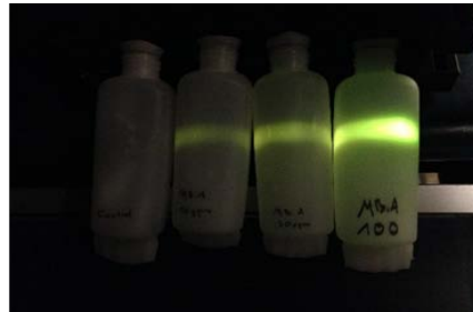
Bottles with and without tracer under ambient light (left) and in laser curtain (right)
