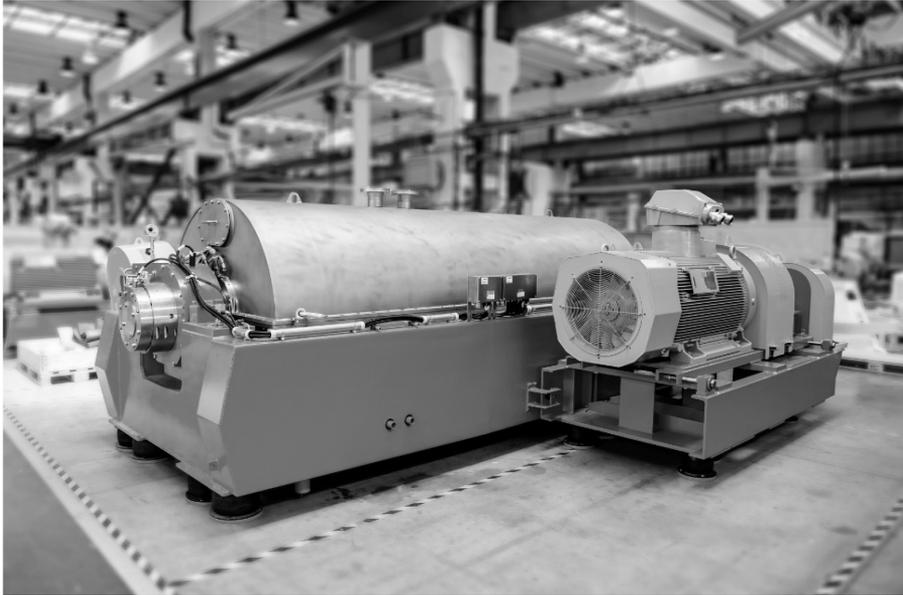
Fig. 3: The ANDRITZ decenter centrifuge CENSOR ACZ with a diameter of 900 mm and a feed rate of up to 6,000 kg/h for highly efficient plastics recycling.
