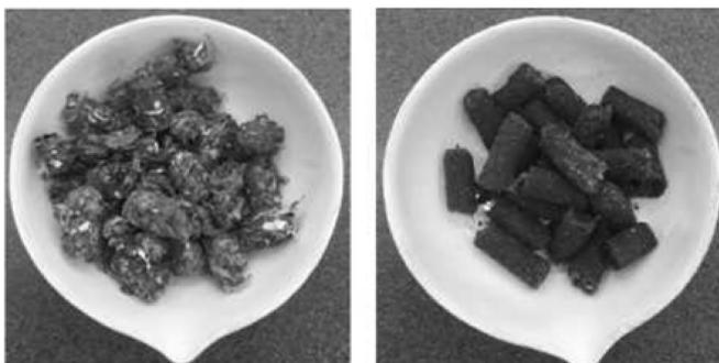
Fig. 4: RDF (left) and bio-fraction (right) pellets.
