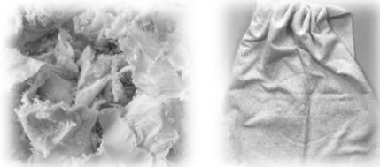
Fig. 5: Collection of selvedges (left) and towel made from recycled PET fibres (right).
