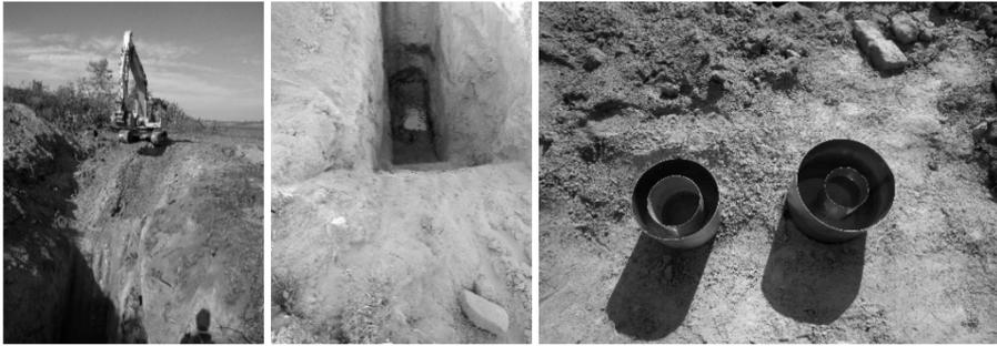
Fig. 1: Soil samples obtained at N77. A spot with high hydrocarbon contamination (up to 40,000mg/kg) was selected based on prior drilling tests. Left and middle: The hole. Right: Infiltration tests on-site with water and rapeseed oil in double ring infiltrimeters.
