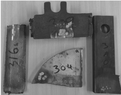
Fig. 4: Picture of the four steel samples (SUS304, SUS309, SUS310 and SUS316) with different thickness of rust or oxide layer. For each sample a subarea was polished for analyses with spark atomic emission spectroscopy.
