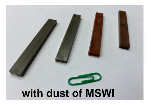
• Tests have shown a significant advantage of the developed composite in terms of strength properties, compared with the analogue material, wood-polymer composite
