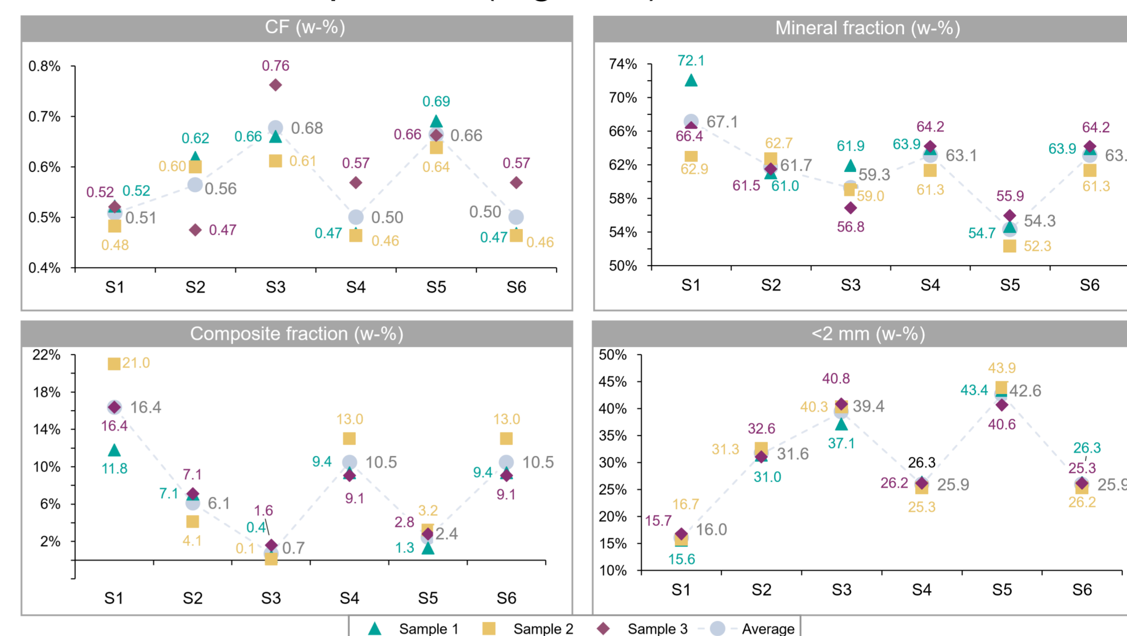
Figure 4. Percent division by weight of four different fractions (CF, mineral, composite and <2 mm) after comminution process.
