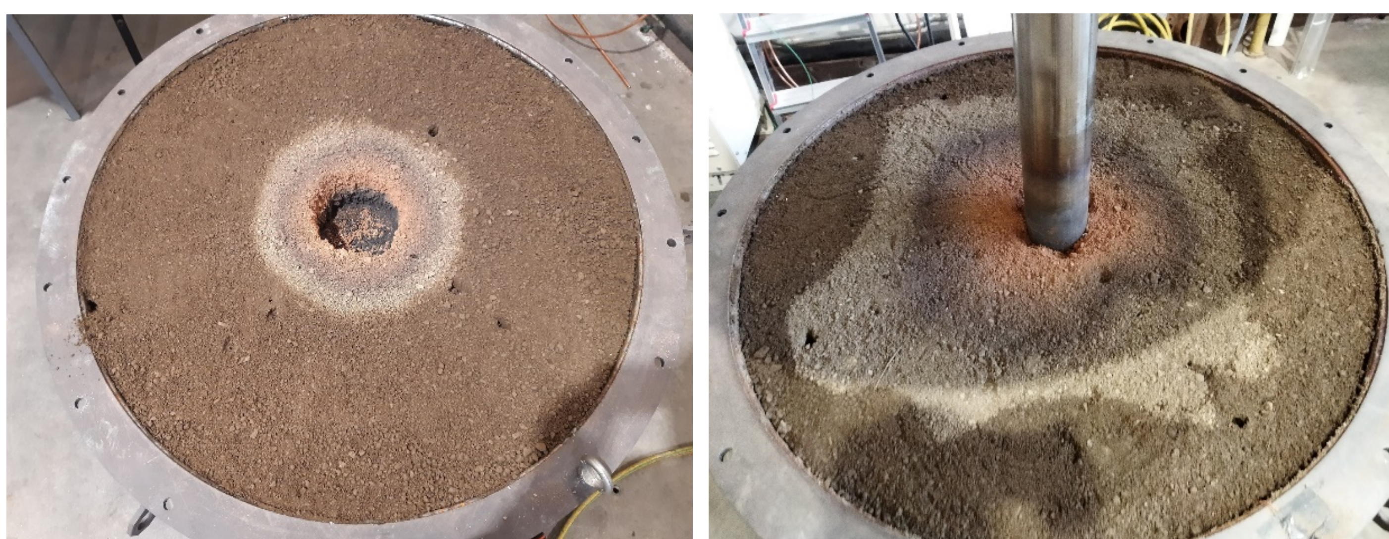
Fig. 2: Surface area of the soil (a) without extraction of soil air, (b) with extraction of soil air.
