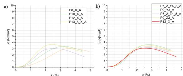
Briquette strength after 48 hr with a) only reducing Portland cement quantity; and b) with Cupola Furnace or Ground Granulated electric arc furnace slag inclusions.
