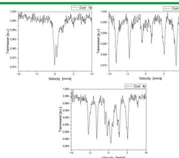
Mössbauer Spectroscopy and ICP-OES of different dust samples was done for foundries of two different foundries and the resulting table of composition.
